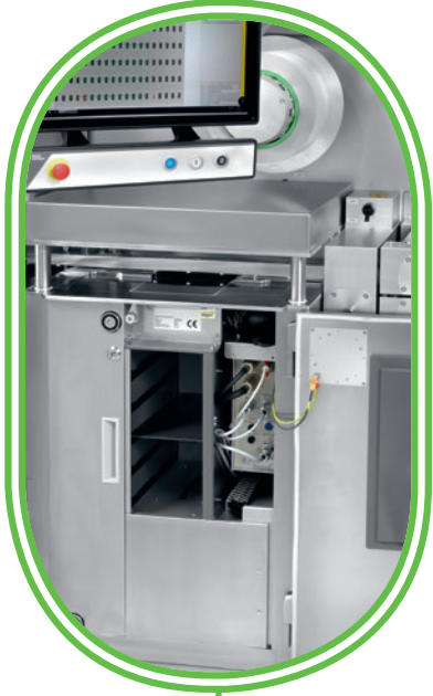
Compact and safe integration of the X-ray module in the Blister Machine SSP2. Convenient operator control via the HMI operator panel.
