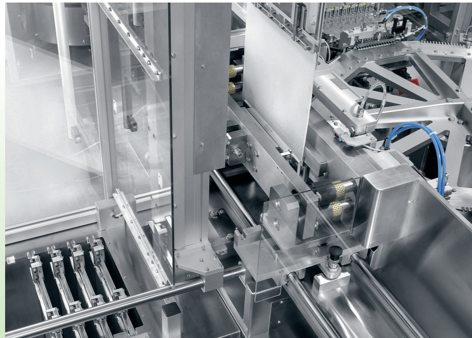
The sponges are punched in parallel from fleece soaked in IgE liquid and then pushed into the caps.
