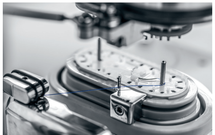
The swaged needle-thread-connection is fastened in a tray. Then the thread is wound on the tray with up to 800 revolutions per minute.
