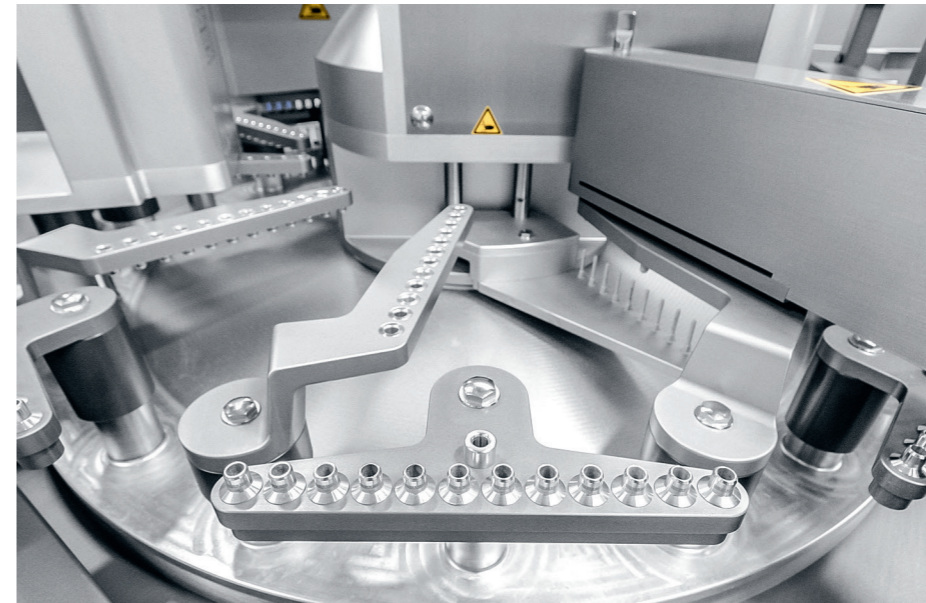
For the dosing of highly cohesive and compressible powders, Micro-Sphere relies on the Modu-C with drum filling technology.
