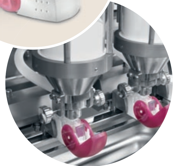
The powder reservoir of the NEXThaler® is filled by means of a high-precision auger doser.
