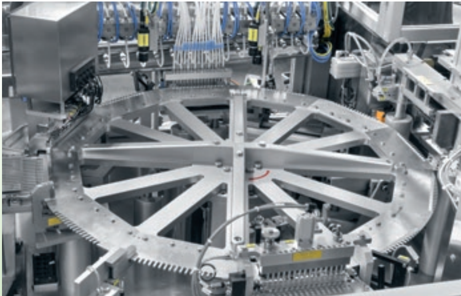
The caps are fed to an intermittently rotating turret, where the sponges are inserted.
