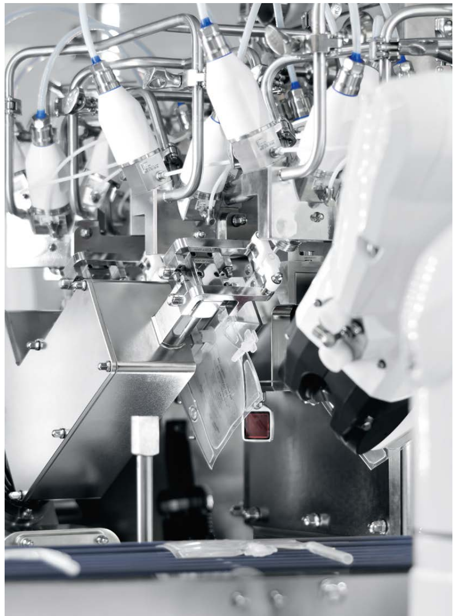
The filling tube and the filling nozzle remain connected until the IV bags are transferred from the machine. This one-time docking principle minimizes the risk of particle entry.
