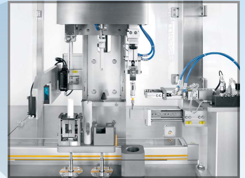
The Assembly Lab is a semi-automatic assembly machine for injection pens and auto-injectors. It is used for the final assembly of devices for small series and clinical studies.
