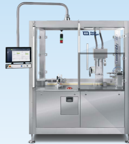
The Assembly Lab is a semi-automatic assembly machine for injection pens and auto-injectors. It is used for the final assembly of devices for small series and clinical studies.
