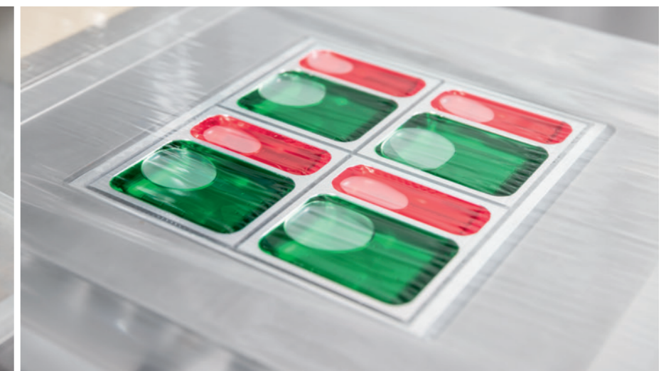
Left: The PVOH film is thermoformed to shape, then the chambers are cleanly filled with various media such as powder, gel or liquid. Right: After water sealing of the top and bottom film, the multi-chamber packs are punched out or cut out.
