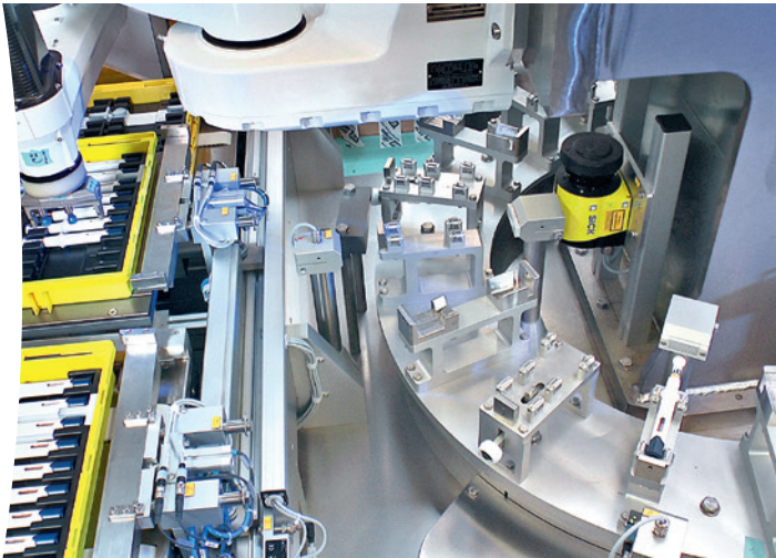
Fully automated product handling for pen labeling
