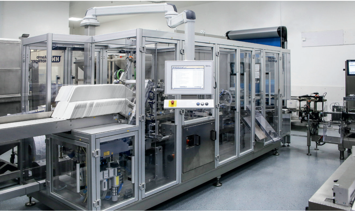
The new packaging line for double bags with its centerpiece: The MKL Cartoner.
