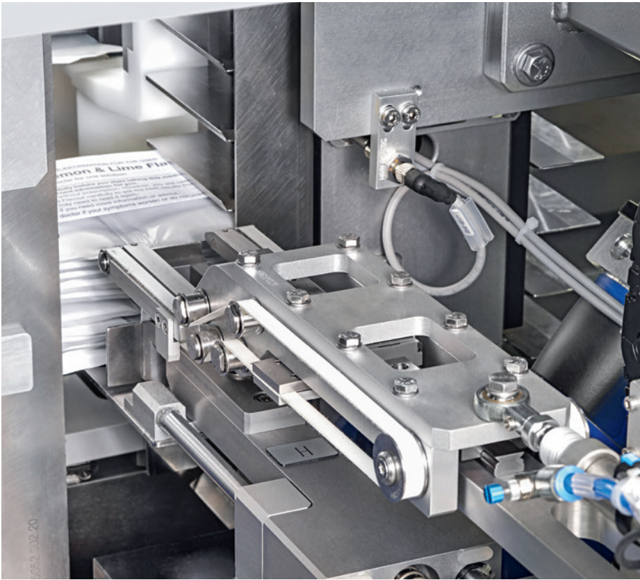
Insertion of double bag stacks into folding carton.
