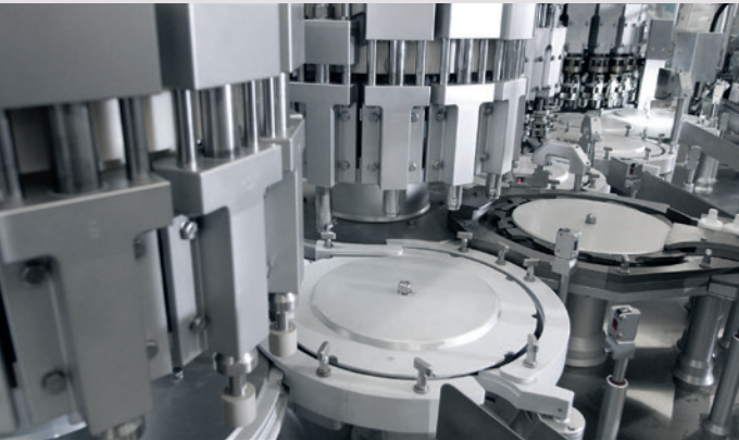
Exactly synchronized processes during drawing and crimping of aluminum shells.
