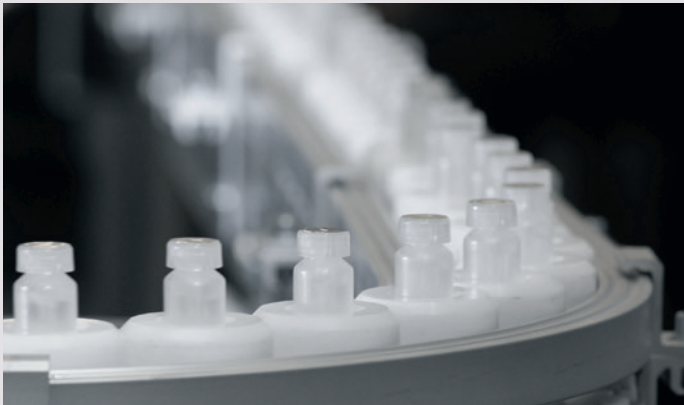
Transfer of liquid cartridges towards the drawing and crimping system.
