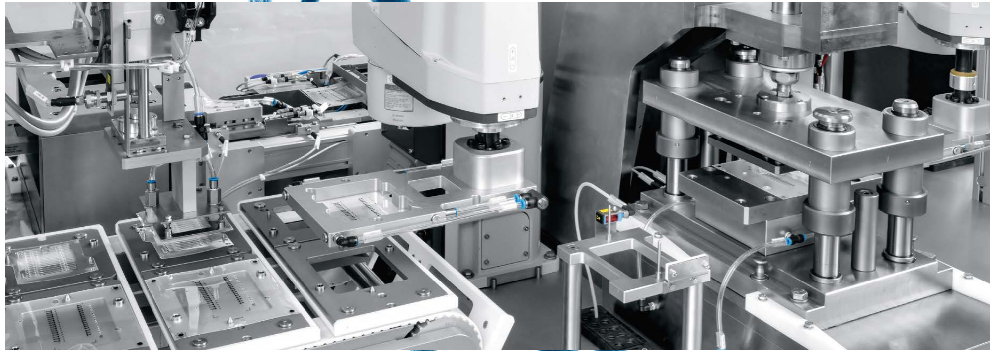
The machine developed by Harro Höfliger precisely joins the two main components of the ScreenTape, which consist of film material: The Printed Layer with its imprinted electrode connections and the thermoformed Process Layer.
