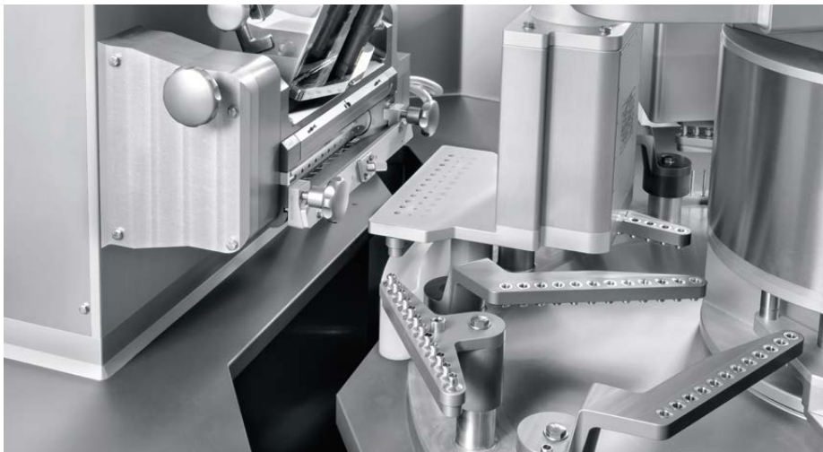
Fully automatic calibration makes processes for capsule filling more reliable.
