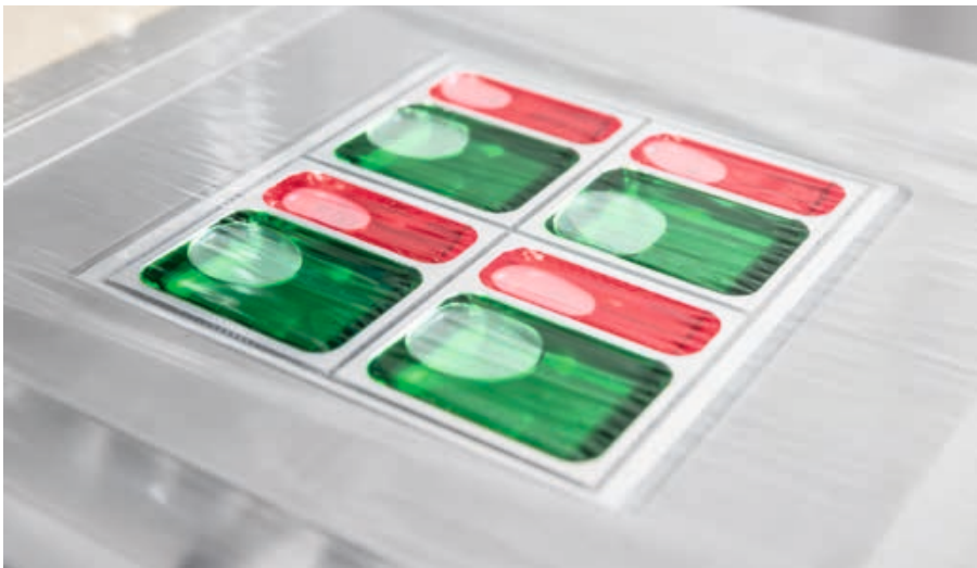
Left: The PVOH film is thermoformed to shape, then the chambers are cleanly filled with various media such as powder, gel or liquid. Right: After water sealing of the top and bottom film, the multi-chamber packs are punched out or cut out.
