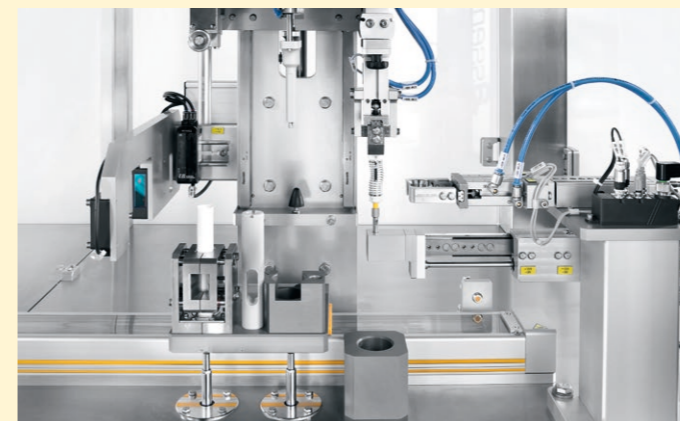
The final assembly of smaller series can be performed on the semi-automatic Assembly Lab system.
