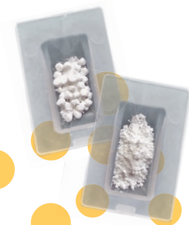
The dry powder before (right) and after pressing into powder compacts (left).
