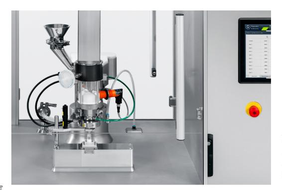
In the auger doser, the powder is stored in a container. The eponymous auger transports it from there to its destination with rotational movements. The principle is suitable, for example, for filling dry powder inhalers.
