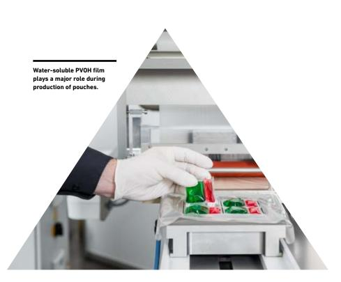
This is where Harro Höfliger's special thermoforming method comes into play: "It is based on our patented continuous forming process in which heat and vacuum are optimally coordinated with each other. By heating the film more slowly, it gains elasticity without high temperatures, and the vacuum required is also reduced. Ultimately, this results in more film thickness, even when it comes to complex designs."
